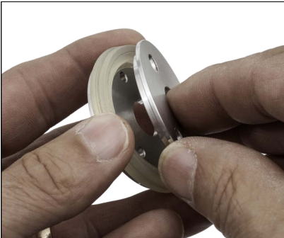
Separate the top and bottom support wheels.
