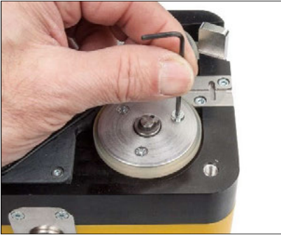
Remove all six M3 countersunk screws.
