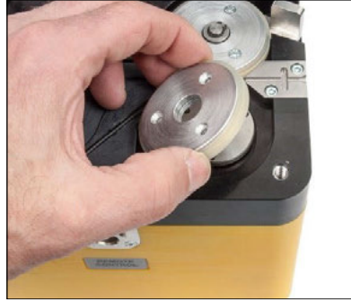
Remove the two wheel assemblies off the drive hubs
