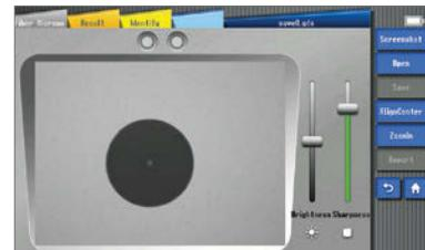
Fiber end tester (peripheral required) is mainly used to test the cleanliness and flatness of the fiber end-face.
