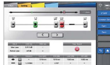
SOLA is an application for the OTDR, designed to simplify the OTDR test process without the need to configure parameters or analysis while parsing multiple complex OTDR curves
