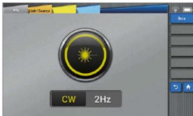
VFL can be used to find direct defect locations in dead zones of fiber testing or to calibrate the fiber core in multi-fiber cables.
