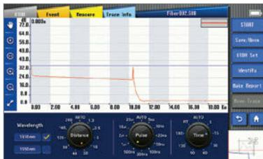
OTDR mode is adopted to measure distance, loss, reflectivity, attenuation and accumulation loss on a fiber optic link.
