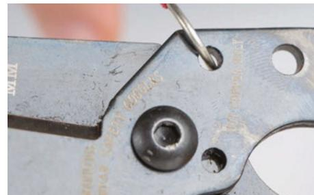
Strips & cuts the most commonly used solid and stranded wires with center conductors from 16 AWG - 26 AWG (1.3 mm - 0.40 mm). This wire stripper features the following:
