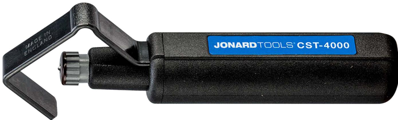
The **PATENTED** CST-1900 and CST-4000 Round Cable Strip & Ring Tools are designed for fast and precise removal of cable jackets from round cables. The CST-1900 removes cable jackets 3/16" to 1 1/8" (4.5 mm to 29 mm) in diameter and the CST-4000 removes cable jackets 3/4" to 1 5/8" (19 mm to 40 mm) in diameter. These round cable strippers feature the following:
